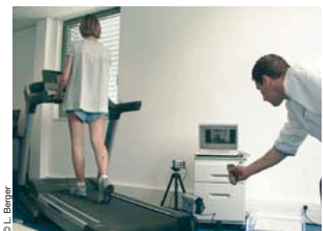
Figure 2. The subjects walked on a treadmill at a constant speed of 3.7 km/h and wore the same model of footwear.
